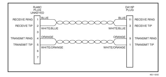
Figure D-2. T1 Line Interface Cable, RJ48C-to-DA15P
